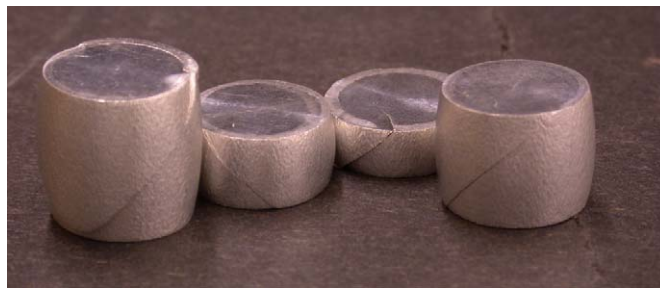
Fig. 4. Deformed specimens with different ratios showing shear fracture.
